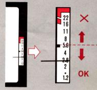
If the battery is good, the meter needle will rest at or below the battery check index. If there is not enough power, it will rest above the index. Replace the battery.
