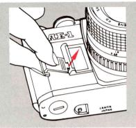
Open the battery chamber cover using the viewfinder cover.
