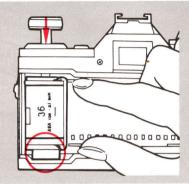
The AE-1 uses color (negative or slide) or black and white film in standard 35mm cartridges. Place the cartridge in the film chamber as shown. Then push the rewind knob down, rotating it until it drops into its normal position.
