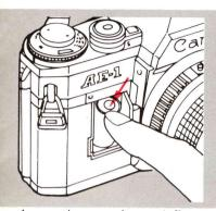
Insert the negative end first. Then push down and insert the positive end. Close the chamber cover.
