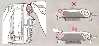
Advance the film once. Check that the film perforations are engaged in the teeth of the film transport sprocket and the take-up spool.
