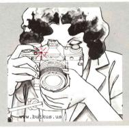
To start the self-timer, press the shutter button. The selftimer lamp will begin to blink. When it stops blinking ten seconds later, the shutter will be released automatically.
