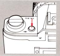
Press the battery check button while looking through the viewfinder. The meter needle in the viewfinder will move.
