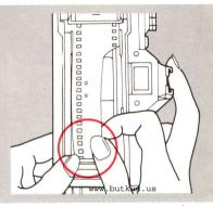
Pull the film leader across the camera and insert it into any slot of the take-up spool.
