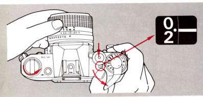
Take several blank shots, releasing the shutter and advancing the film, until the frame counter reads "1" (the dot following zero). While doing this, keep an eye on the rewind knob. If it rotates in the direction of the arrow, the film is loaded correctly.
