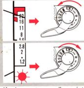
If the meter needle points to the red zone at the top of the scale or if the red LED (Light-Emitting Diode) blinks below the scale, turn the shutter speed dial as shown. Otherwise, exposure will be correct at the shutter speed you have set.
