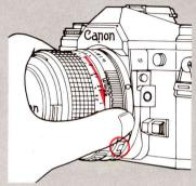
Make sure the lens release button has popped out. Otherwise, the lens will not work properly. DO NOT press the lens release button while mounting or it will not pop out.
