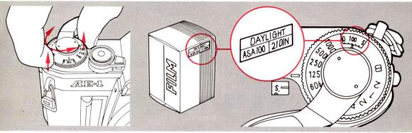
Lift the knurled ring around the shutter speed dial and turn it until the ASA speed of your film is aligned with the green index. This is absolutely necessary for getting correct exposure.
