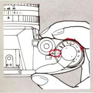
Set a shutter speed by turning the shutter speed dial until a number from 60 to 1000 is aligned with the index.
