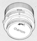
Remove the rear lens cap by turning it in the direction of the arrow until it stops and pulling it out.
