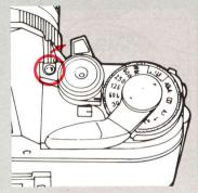
Push the self-timer lever forward to uncover the self-timer lamp.
