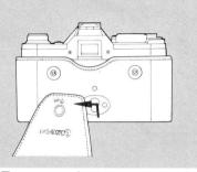
To remove the top cover, turn it down, then push it straight up and out. Turn the lens' focusing ring to infinity  $(\infty)$  for closing the top cover.
