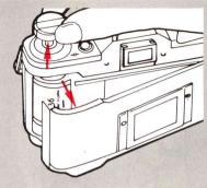
You can tell you have reached the end of the film by the frame counter and the film advance lever. Either the film advance lever will not turn at all or it will not turn all the way. First press in the rewind button. You may immediately let go of it.
