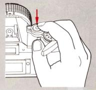
Turn the shutter button lock lever to "A".
