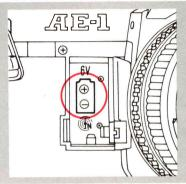
Load one new battery so that its poles are in the directions indicated by the diagram inside the battery chamber.
